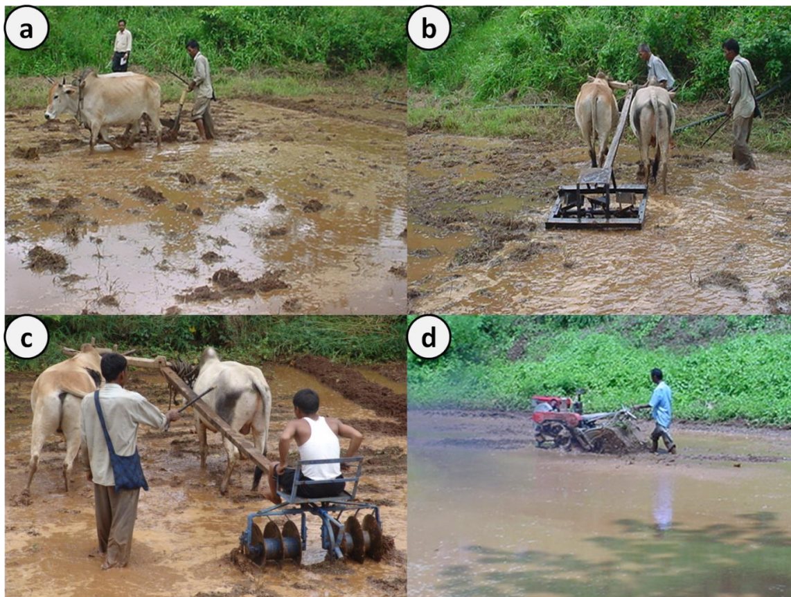
Figure 1. Puddling operation by a) Traditional country plough, b) animal drawn rectangular blade puddler, c) animal drawn disc harrow and d) power tiller operated rotavator
